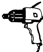
Fig. 8.11: Impact wrench with pneumatic drive
