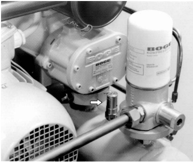
Fig. 9.4: Safety valve on combined compressed air-oil receiver of an oil-injection cooled screw compressor
