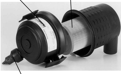
Fig. 3.43: Intake filter with paper insert
