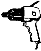
Fig. 7.4 : Drive screw powered by compressed air
